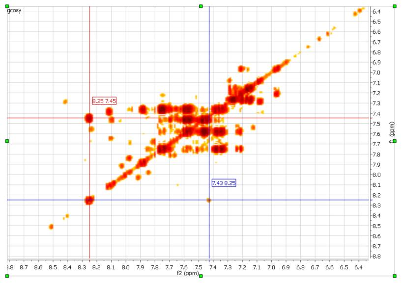
Select *View→2D Plotting Method→Contour Plot* or right mouse button click. Contour drawing on the fly is slower. Do this after data processing.
