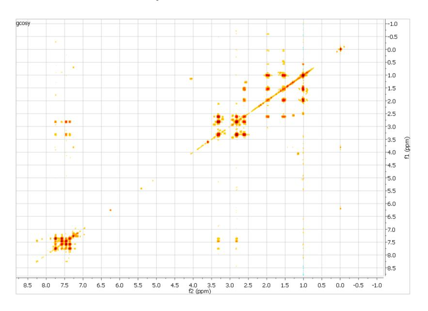
Turn on *Processing→Reduce t1 noise.* In this case, the improvement is significant, but be cautious with artifacts. To turn off t1 noise correction, toggle off *Processing→Reduce t1 noise*
