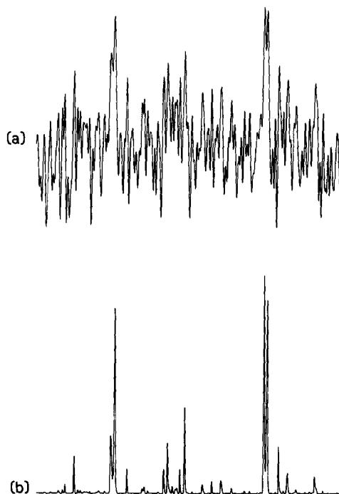
FIG. 2. Simulated spectra of an AX spin system produced by (a) a conventional FT of the first 256 points of the same FID as used in Fig. 1 but after adding noise having a standard deviation equal to 71% of the first point and using matched filtration; and (b) a MEM reconstruction using the same data.
