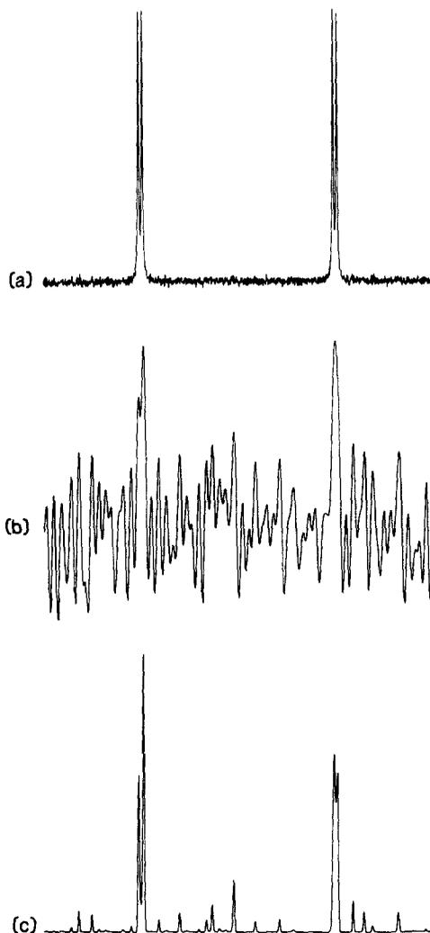
FIG. 1. Simulated spectra of an AX spin system produced by (a) a conventional Fourier transform (FT) of a 1024 point FID after adding noise having a standard deviation equal to 1% of the first point; (b) a conventional FT of the first 128 points of the FID after adding 50 times more noise; and (c) a MEM reconstruction using the same data as in (b).
