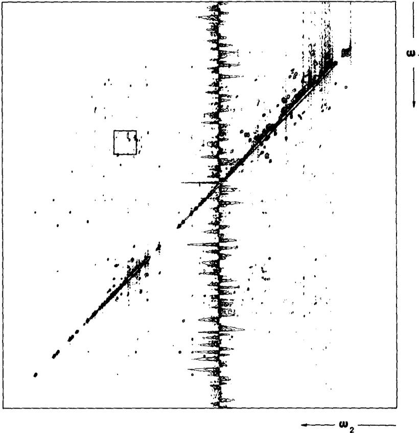
FIG. 4. A NOESY spectrum acquired at 400 MHz on a Bruker AM400 instrument of the protein basic pancreatic trypsin inhibitor (BPTI) in  $\text{H}_2\text{O}:\text{D}_2\text{O}$ , 9:1, v/v. The  $\text{H}_2\text{O}$  signal was suppressed by irradiation during the relaxation delay. There are 2048 points in  $\omega_2$  and 1024 points (zero-filled from 512 points) in  $\omega_1$ . The square shows the region which is expanded in Fig. 5.
