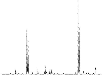
FIG. 3. A simulated spectrum of an AX spin system produced by a MEM reconstruction using 128 points exponentially sampled out of 256 points of the same FID as used in Figs. 1b and 1c. All spectra in Figs. 1-3 have the same digital resolution.
